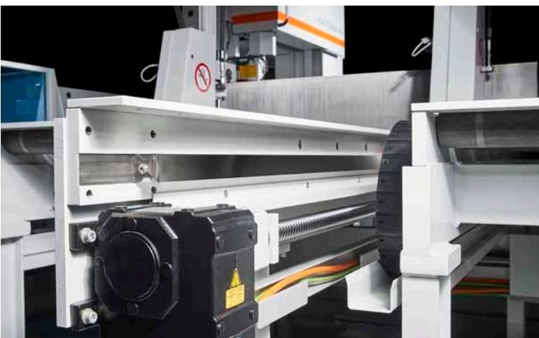
Linear guide unit featuring backlash-free carriage adjustment
