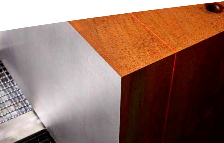
Laser lamp for projecting the cutting line onto the workpiece
