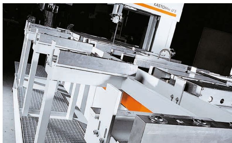
Outer table expansion for processing large sized workpieces
