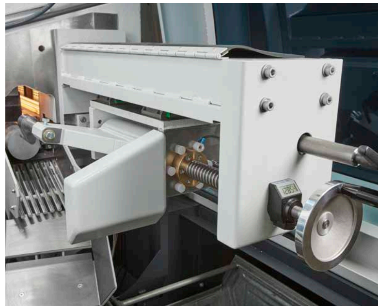
Manually adjustable measuring stop, e.g. with a cut piece length of 1,000 mm
