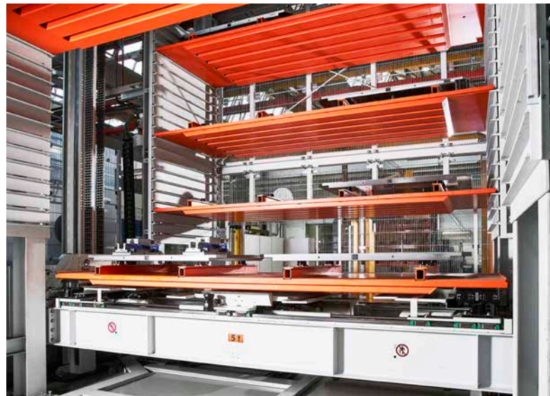
Tower storage with overhead gantry crane for pre-buffering for the CNC metal-cutting machines
