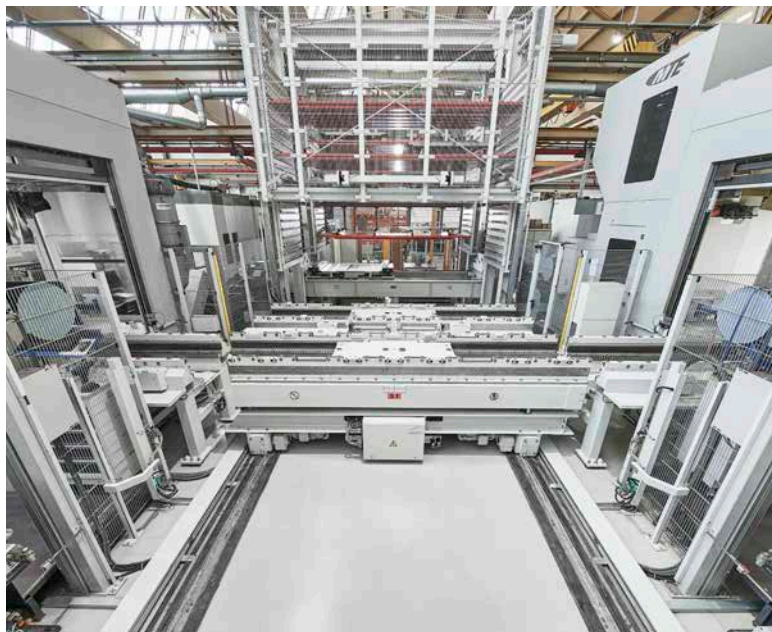
Dual loading table for feeding the CNC machining centres
