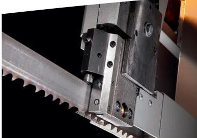
U-shaped tape guide head with band free lifting device.
