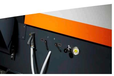
Coolant hose for cleaning the work area / clamping force regulation
