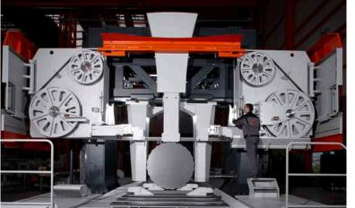
Rigid welding construction in horizontal position with pretensioned linear guides. Bandsaw blade guides with closed supply system. Integrated tool control sensors.
