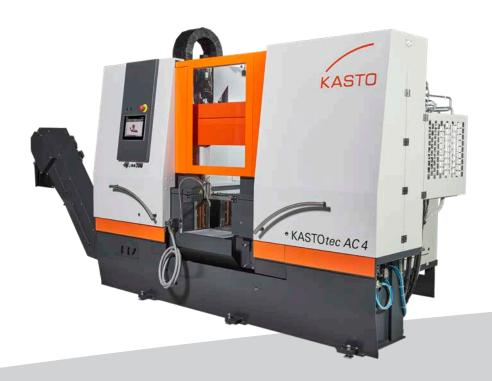
KASTOtec AC, the heavy-duty, high-performance automatic band saw with horizontally parallel moving sawband, for cutting solid material, profiles and pipes of all qualities, including difficult-to-machine materials such as titanium, Hastelloy, Inconel, etc.
