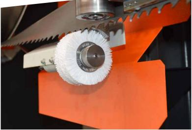
Self-adjusting, motor-driven chip removal brush
