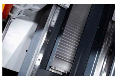
Two linear guide units per column with six play-free adjusted carts each per unit guarantee high rigidity, maximum damping and cutting precision.
