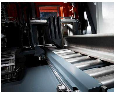
Hydraulic bundle clamping device including closing limiter
