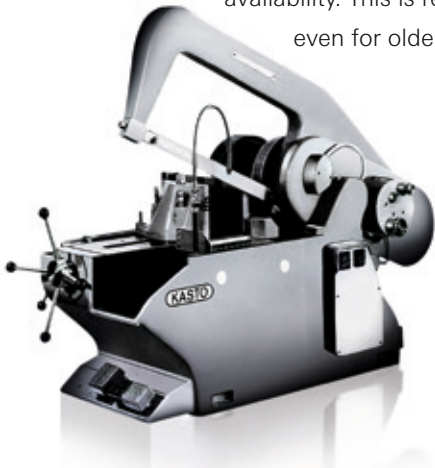
Still in use in many places: KASTO EBS hacksaw from the sixties.
