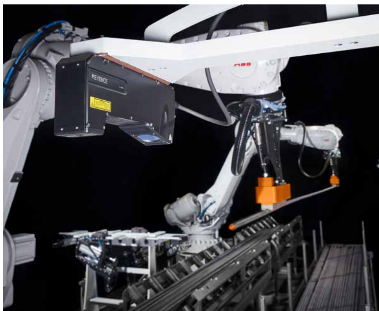
Bar removal with a magnetic gripper using KASTOpick bar
