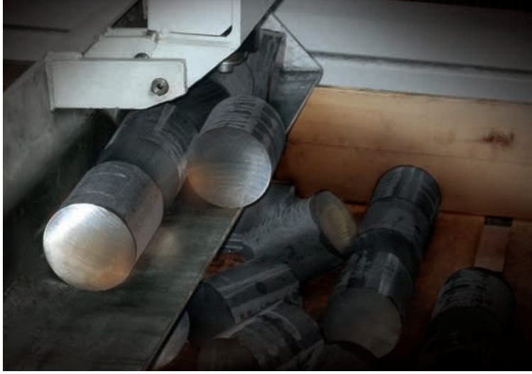
Low noise depositing of heavy cut-off pieces ...
