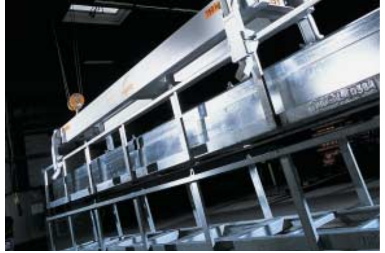
Universal : With the patented gripper technology, even customer-specific transport containers can be economically transported and restacked
