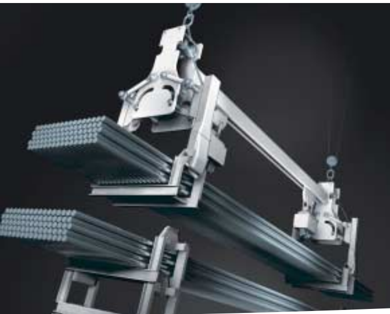
Magnetic : Stacking cradles can be safely manipulated with the UNIBLOC F magnet spreader beam
