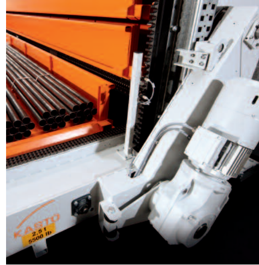
Lifting beam with bar stock cassette and lift motor.
